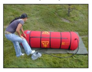
6. Pump the foot operated air pump to begin inflation.
