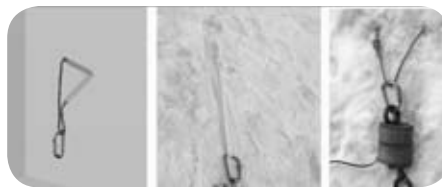
Figure 13 (left and middle) strongest orientation; (middle) strongest orientation and material-vertical 1" tubular webbing single loop; (right) weakest of the three, but still strong enough*.
